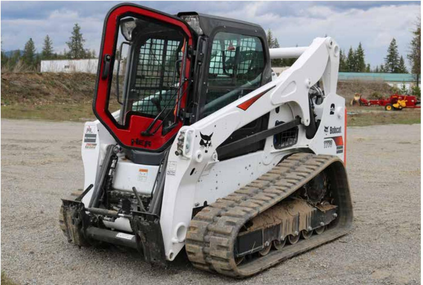
Step-up the safety on your skid steer with a UL752 Level 1 ballistic door better known as the Defender Ballistic Door. Whether you are operating a hammer, auger, mower, mulcher, or a log processor you can feel secure in knowing there is a 3/4" bullet resistant door in place, to help protect your **BIGGEST ASSET - YOU!**
